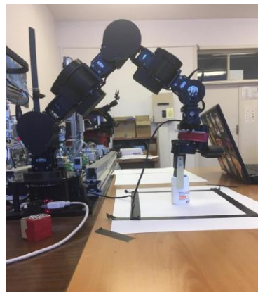
Fig. 5.8 Laboratory testing of the 7DOF robotic manipulator using boxes with variously colored.
