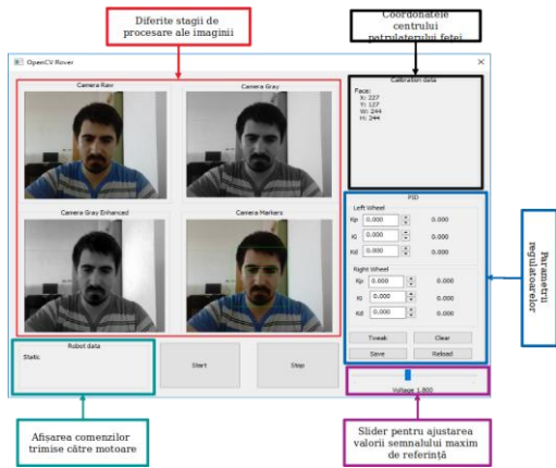
Fig.5.1 Laboratory testing of the navigation structure for the complex autonomous system SAC-SI using the head movements of a person: a) graphical interface, b) the real time testing of complex autonomous system SAC-SI
