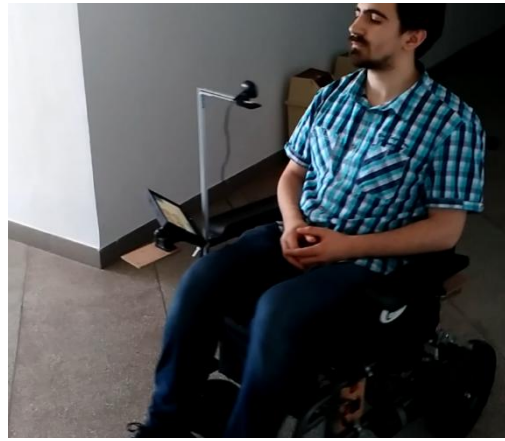
Fig.5.1 Laboratory testing of the navigation structure for the complex autonomous system SAC-SI using the head movements of a person: a) graphical interface, b) the real time testing of complex autonomous system SAC-SI
