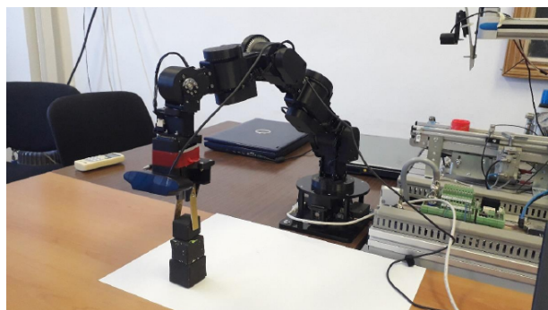
Fig. 2.15.4 The initial and final phase in the case of arranging the objects in a stack in order of their size, from the largest to the smallest.
