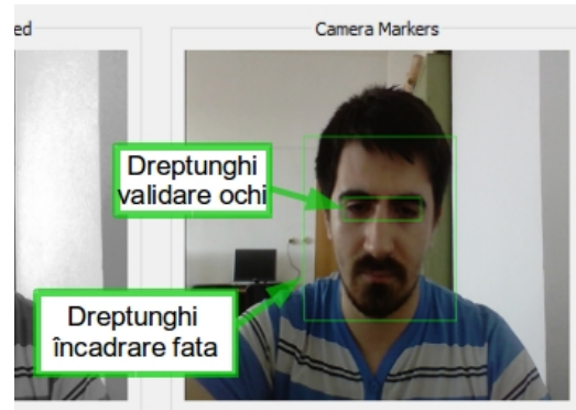
Fig. 2.13.3. Example of valid quadrilateral - which fits both the user's face and his eyes
