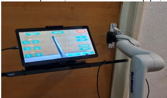
Fig. 4.1.3. Webcam mounted on the final effector and the image displayed on the interface
