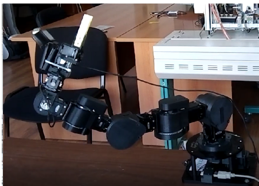
Fig. 1.13.2 Manipulator Cyton Gamma 1500
