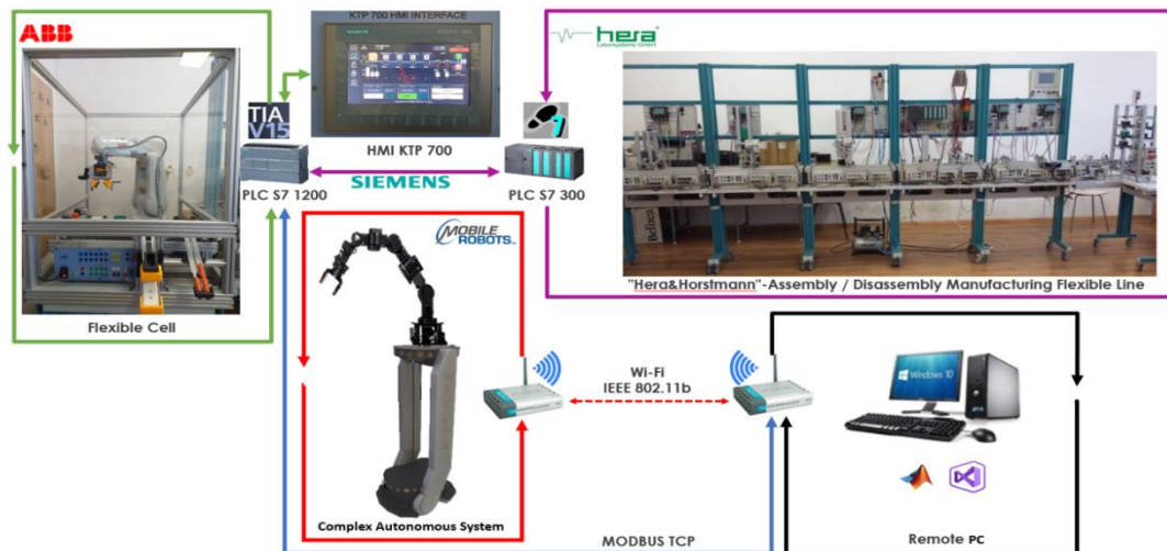
Figure 1 SAC control structure consisting of A / D / R line, CF manufacturing cell and SAC-ARP
